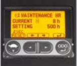
Planned maintenance hour meter notifies operators of the need for routine maintenance and service via the digital display monitor. The service intervals are programmable.
