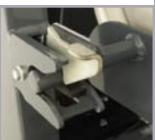
One-touch LP tank bracket latch with rubber grommet is designed to unlatch/latch the LP tank in one motion, while preventing noise caused by truck vibration as it travels over uneven surfaces.
