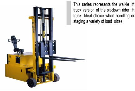
Full system filtration prevents contaminants from entering the hydraulic system. Pressure compensating flow control valve at base of lift cylinder regulates lowering
