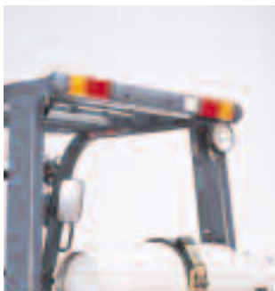
High mount rear combination lights are integrated into the overhead guard, making stops and turns highly visible in the workplace.
