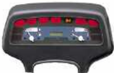
Swing Lock Cylinder indicator light informs operators when SAS is engaged, making them aware of SAS's role in maintaining stability.
