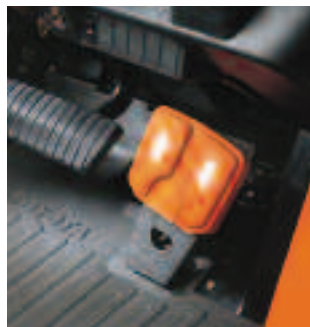
Optional EZ Pedal enables an operator to quickly change travel direction without taking a hand off the steering wheel or hydraulic controls.
